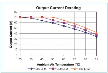
Figure 20 — Maximum output power derating vs ambient air temperature. Longitudinal airflow, Board and junction temperatures <125 °C. Tested with IBC evaluation board IB048Q096T70N1-CB
