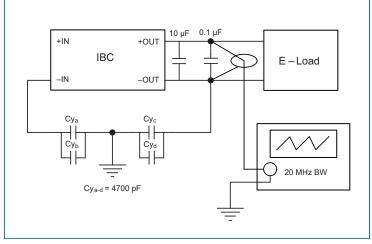
Figure 23 — Test circuit; output voltage ripple
