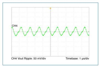
Figure 16 — Output ripple; Nominal line, full load
