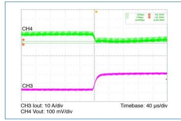
Figure 11 — Load transient response; nominal line Load step 75–100%
