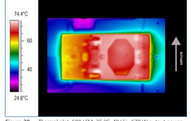
Figure 28 — Thermal plot, 600 LFM, 25 °C, 48 Vin, 670 W output power
