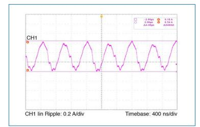
Figure 5 — Input reflected ripple current at nominal line, full load. See Fig 22 for setup.
