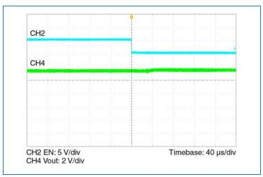
Figure 18 — Three module parallel array test. Vout change with two modules operating and a third module enabled. Nominal Vin, lout = 140 A
