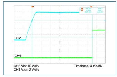
Figure 6 — Turn on delay time; V<sub>IN</sub> turn on delay at nominal line, 15% load
