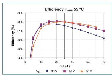
Figure 2 — Efficiency vs. output current, 55 °C ambient
