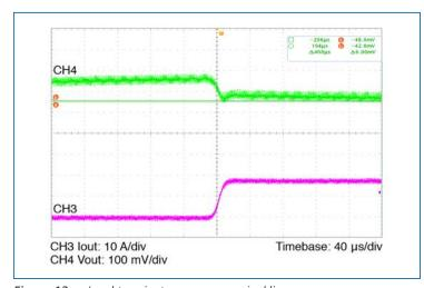
Figure 13 — Load transient response; nominal line Load step 0-25%; 10 Aldiv
