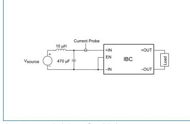
Figure 22 — Test circuit; input reflected ripple current
