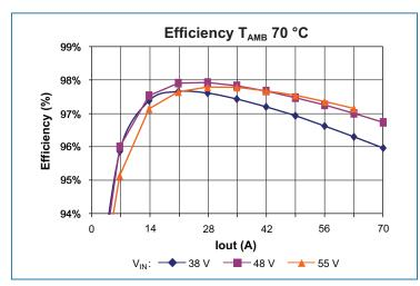
Figure 3 — Efficiency vs. output current, 70 °C ambient
