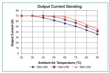
Figure 19 — Maximum output power derating vs ambient air temperature.
