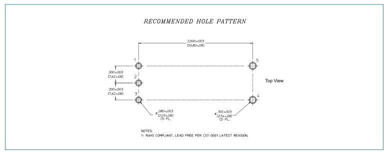
Figure 33 — IBC PCB recommended hole pattern
