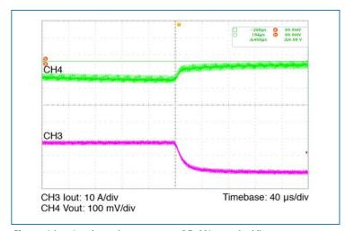
Figure 14 — Load transient response; 25–0%; nominal line
