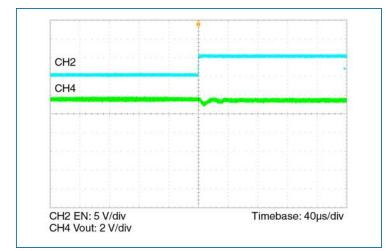
Figure 17 — Three module parallel array test. Vout change when one module is disabled. Nominal Vin, lout = 140 A
